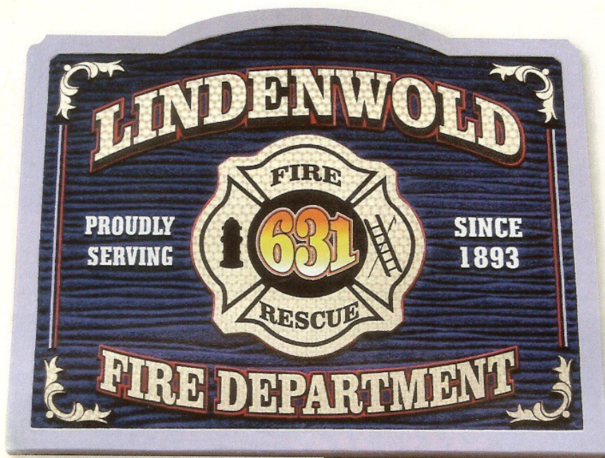
Bordi created this project from 1 1/2" HDU, which was sandblasted by hand to add faux wood grain. The sign was painted with 1 shot, and the lettering was finished with SignGold.
